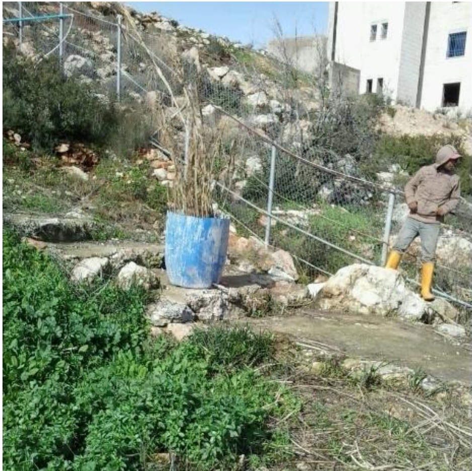
Photo 3. Plastic barrel to calculate the quantity of evapotranspiration, photo date (15/January, 2016)/Qarawit Bani-Zeid village/ Palestine
