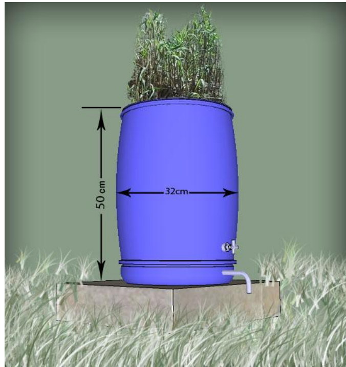
Photo 4. A mini pilot of the constructed wetland plastic barrel to calculate the quantity of evapotranspiration
